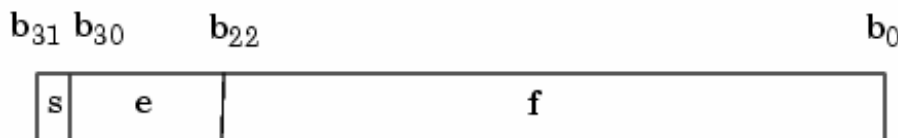
Figure 1.3 IEEE 754 Floating Point Number construction for 32 numbers
